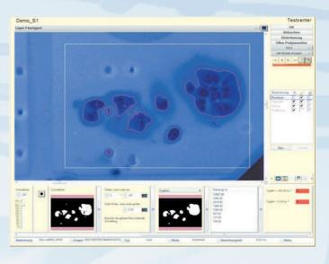
In order to detect conformal coating defects, it is necessary that the coating material has an UV trace. The product has to illuminate with UV light and using the fluorescent light for the inspection.
