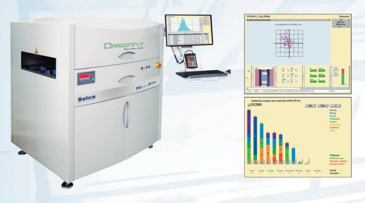
The combination of multi-colored LED lighting and color scan camera offers a deep inspection of the solder joint meniscus and the shorts detection, while the full scan acquisition of the PCB surface and not only of the components allows the solder balls detection.
