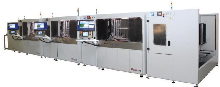
**pass-through** version, with dedicated loaders and unloaders, it is the operator-free test solution for the manufacturing environment.
